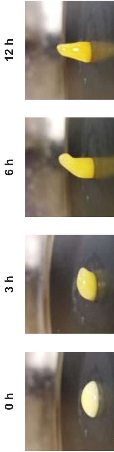
Figure 3.6. Photograph images of 75 \mu l of resultant pollen pipetted onto a platform show that the suspension consistency transforms from a wet sand slurry to an agar-like consistency with increasing KOH incubation from 0 h to 12 h.
