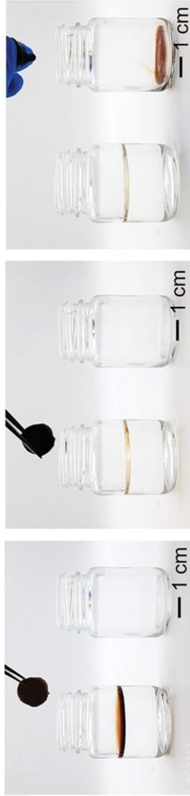
Figure 5.19. Absorption, removal, and squeeze-mediated release of motor oil from contaminated water sample by using a pollen sponge. 304
