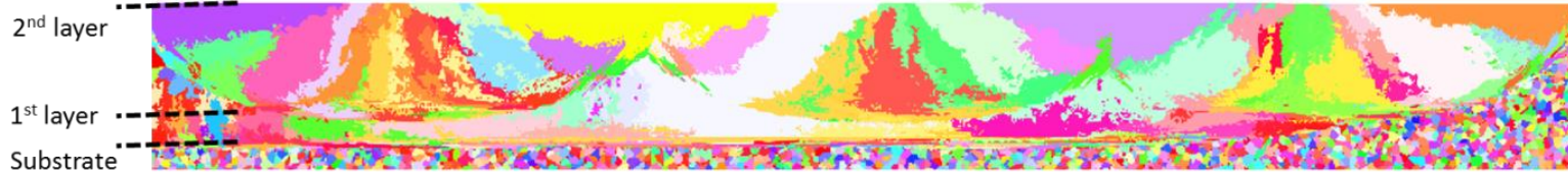
Figure 4-9 Top: Simulated grain structure in 3D with 3 combined tracks per layer for 2 layers, bottom: cross section of two planes showing the grain orientations. IPF-maps shown have the crystallographic orientations relative to the building direction.
