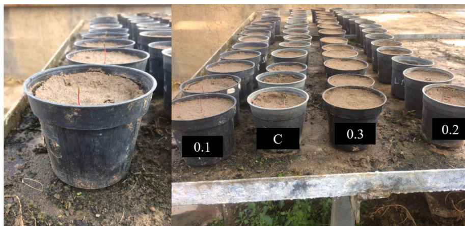
Fig. 14. Germination of MICP treated samples with 0.1 and 0.2 M cementation solution as well as control.
