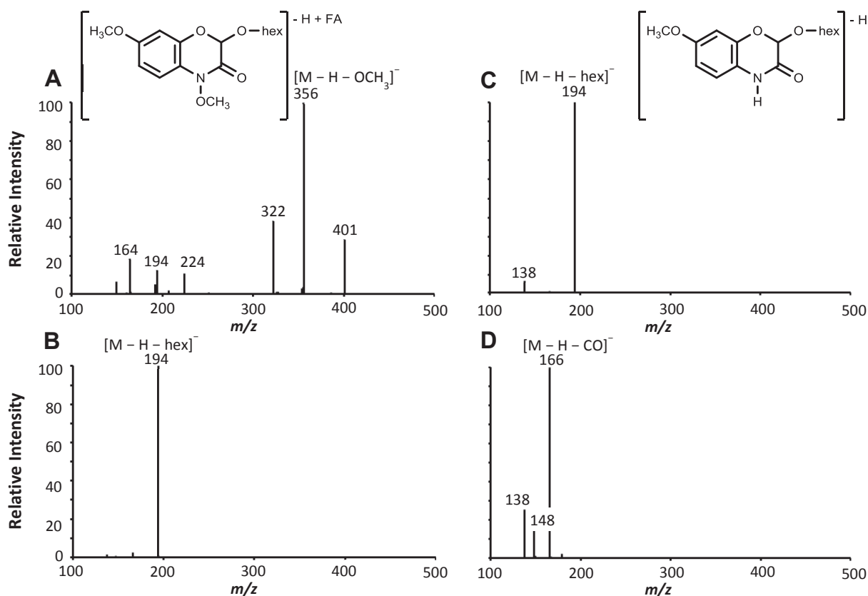
Figure 3.4. Fragmentation spectra of (A) the formic acid adduct of HDMBOA-hex m/z 432, a methyl derivative, in MS 2 ; (B) its most intense product ion m/z 356 in MS 3 ; (C) the deprotonated molecule HMBOA-hex m/z 356, a lactam, in MS 2 ; and (D) its most intense product ion m/z 194 in MS 3 . hex, hexose.
