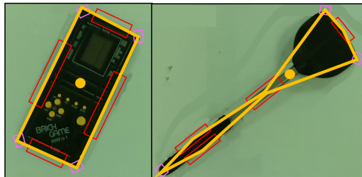
Figure 6. Feature detection and determination of abstract shape: The red boxes show the detected straight edges and the pink boxes show the detected corners. The yellow line shows the concave hull of all these detections, which provides the estimated perimeter and enclosed area of the object. The yellow circle shows the estimated centroid of the object derived from this concave hull.
