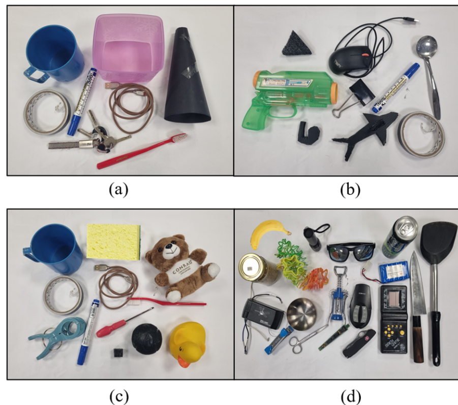
Figure 16. (a) Similar object set used for GPP testing [18]. (b) Similar object set used for DexNet 2.0 testing [19]. (c) Similar object set used for GG-CNN testing [20]. (d) Object set designed by this study for algorithm testing.
