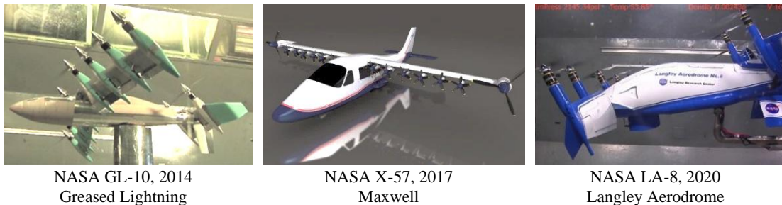
Figure 2.6: NASA Distributed Electric Propulsion prototype demonstrator aircraft [64–66].
