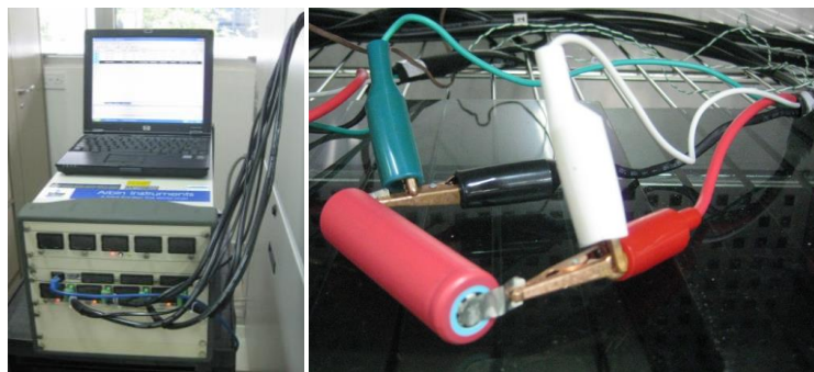
Fig. 2.5. The battery testing system.
