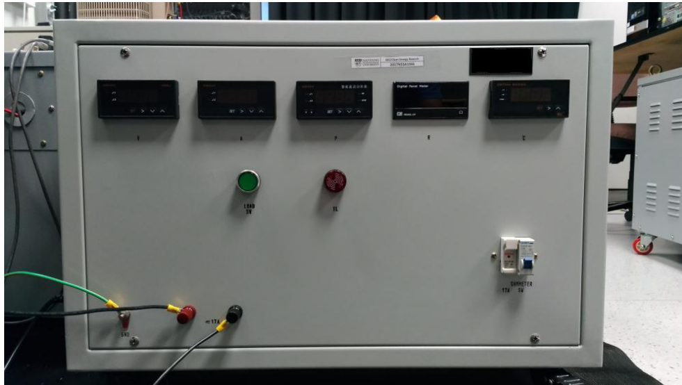
FIGURE 4.18: Adjustable load resistor box.
