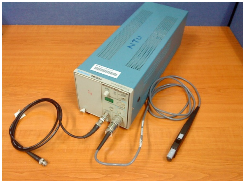
Figure A-3: Current Probe & Current Probe Amplifier
