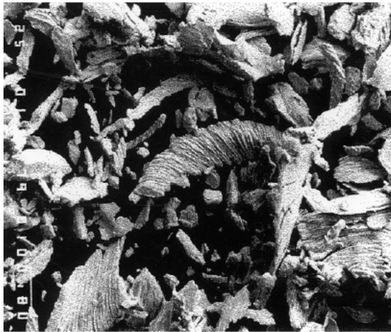
Figure 2.39: Ribbon shaped particles formed by micro cutting (Rigney, 1992)
