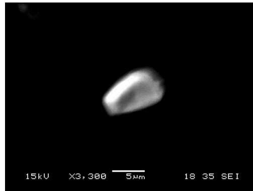
Figure 5.22: Irregularly shaped Wear Debris obtained at 150 mins
