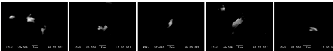
Figure A.13: SEM pictures of wear debris particles obtained after 90 mins for Analysis Experiment
