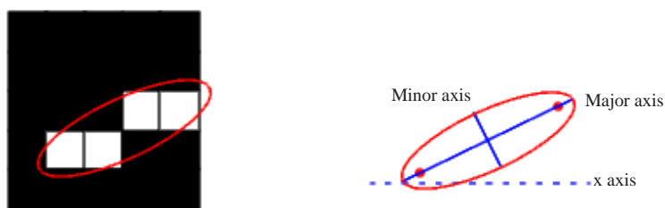
Figure 4.27: Axes and orientation of the ellipse
