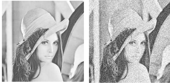
(a) 256 \times 256 image of 'Lena' (b) Noisy version of Lena ( SNR = 5.63db )
