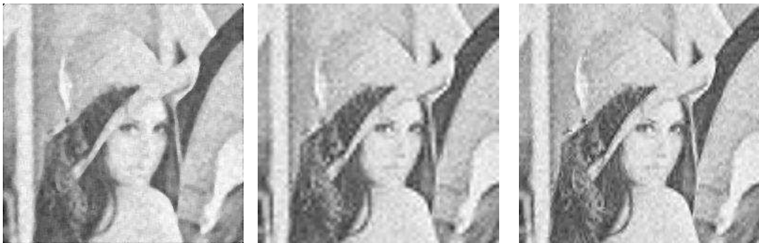
(a) Denoised using Median Filter ( SNR = 10.32db ) (b) Denoised using VisuShrink ( SNR = 10.33db ) (c) Denoised using BayesShrink ( SNR = 11.31db )
