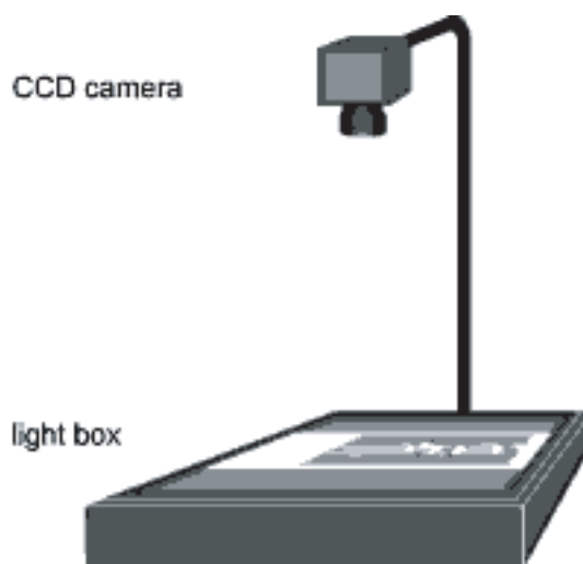
Figure 2.6: Principle of the CCD array camera
