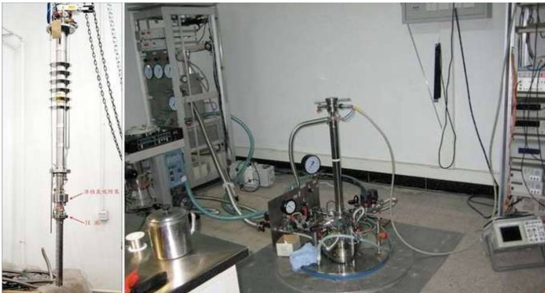
Figure 3.10 3He cryostat (Oxford, HelioxTL, Top-loading, Base T=250 mK with a 17 T magnet) used for measure the superconducting in MoTe 2 .
