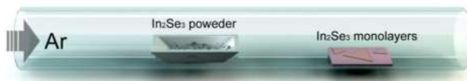
Figure 7.1 Schematic diagram of the PVD system used for the preparation of \text{In}_2\text{Se}_3
