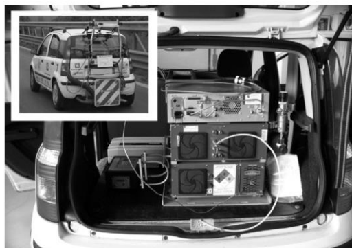
Figure 2-4: Passenger car instrumented with PEMS (Franco et al. 2013)
