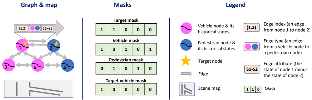
FIGURE 4.4: Processed data. Left , the directed edge-feathered heterogeneous interaction graph (top) obtained after processing and the map (bottom). Middle , the mask vectors. Right , the legend of this figure. The interaction graph is constructed via a close connection strategy, where each node is only connected to its neighboring nodes via directed edges. A directed edge is identified via its edge index and contains edge type and edge attribute.
