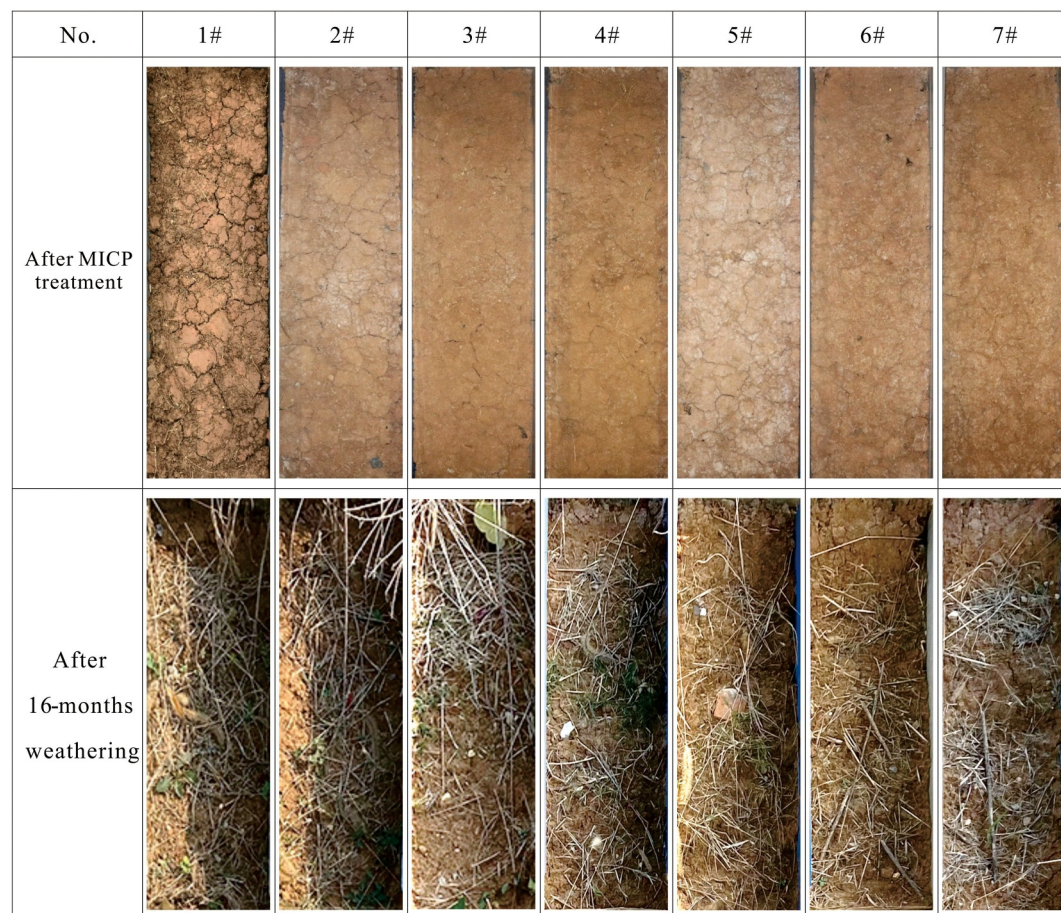
Figure 2. Pictures of test slopes after MICP treatment and after 16-month weathering.
