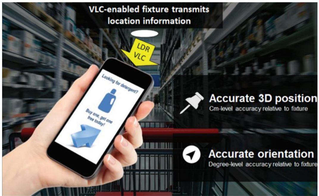
Figure 2.8. Illustration of VLC based indoor positioning [8].
