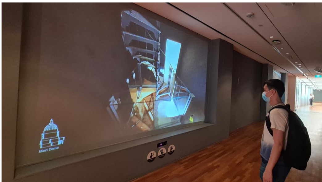
Fig. 68. The installation at the NGS uses Kinect to read the body's movement to translate into navigation in the software.
