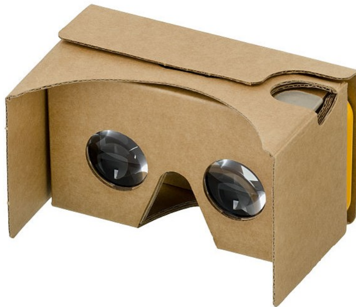
Fig. 21. An example of a Google Cardboard with a smartphone inserted inside the cardboard visor. It was Google's way of introducing VR to the masses with an inexpensive cardboard container and plastic lens.
