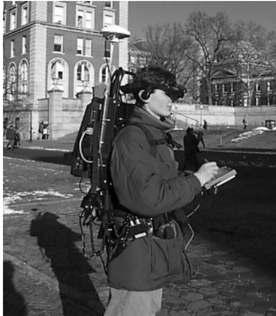
Fig. 16. The Touring Machine consists of a backpack holding the computing system, the HMD, a tablet, and a stylus.
