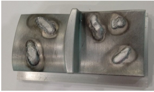
a) Freeform component with small weld beads
