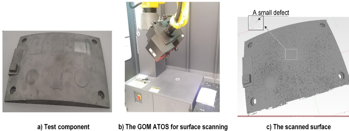
Figure 4.13 Data acquisition from a test component
