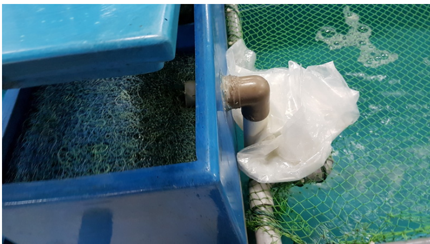
Figure 2.5: the inside of the custom-made filter units in the Diamond Koi farm. The net-like plastic structure in the tank are physical filters, and the water is pumped through it via the PVC pipes shown on the right.
