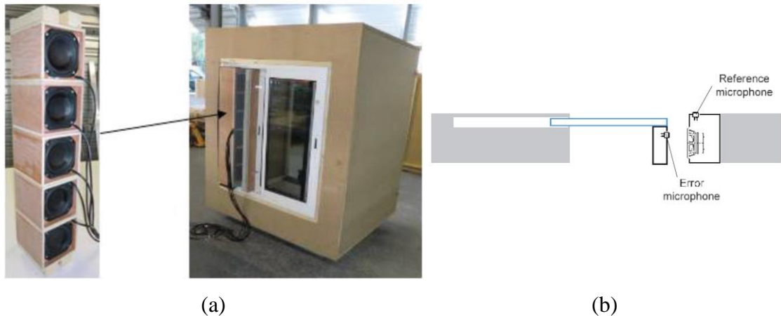
Figure 2.5: (a) Active control units in a sliding window configuration, and (b) a cross-sectional view of the system [Carme et al., 2016b, 2016a].
