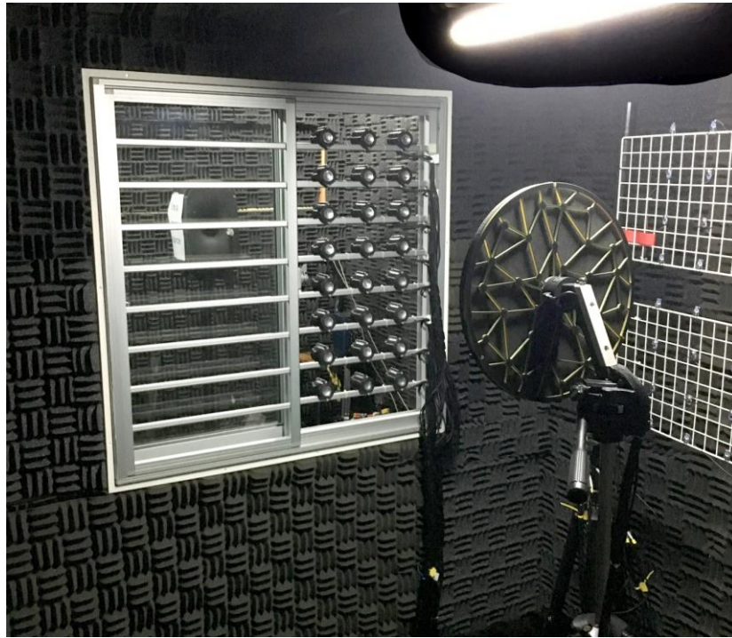
Figure 5.4: Image of the acoustic camera placed 1 m from the window in the interior of the test chamber (Image has been enhanced for clarity).
