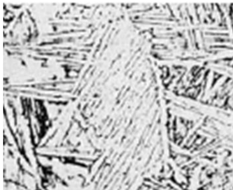
\alpha+\beta alloy: Acicular \alpha+\beta alloy in Ti-6Al-4V
