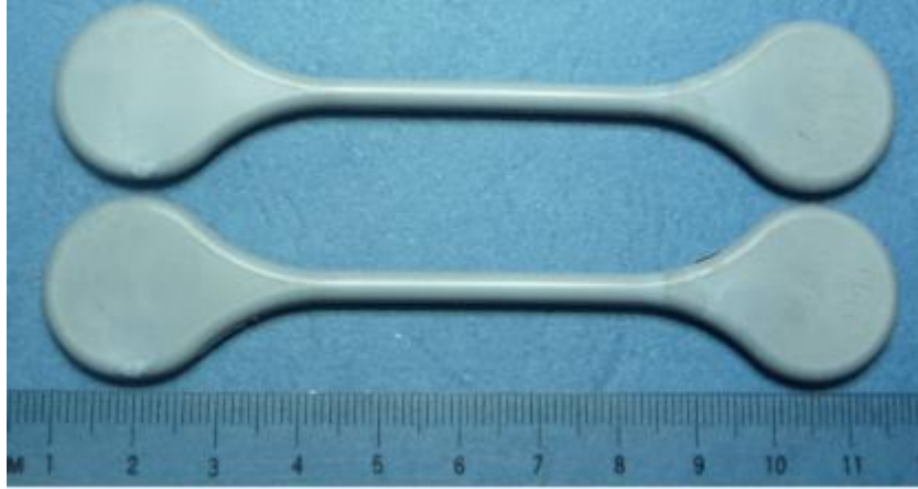
Figure 3.10 CP-Ti tensile components after solvent debinding.
