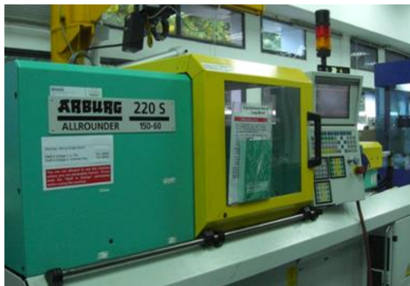
Figure 3.7 Arburg 220S 15 ton PIM machine.
