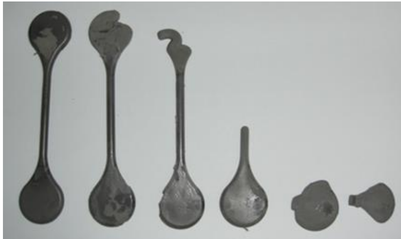
Figure 3.9 Progressive filling of cavity during injection moulding.
