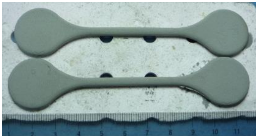
Figure 3.12 Tensile components after solvent and thermal debinding.
