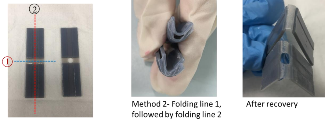
Figure 59. Crossfolding for 0.1 mm sample
