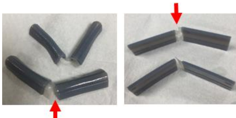
Figure 60. Fracture for 0.1 mm sample
