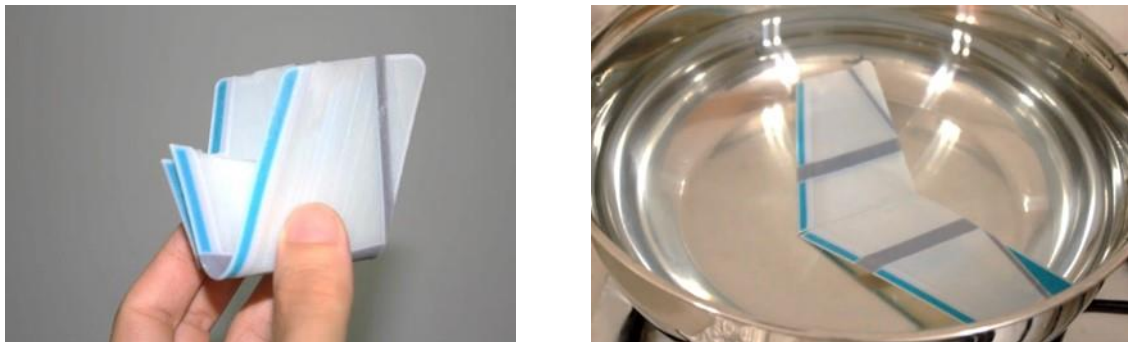
Figure 19. Multi-folding glider (a) before heating and (b) after heating
