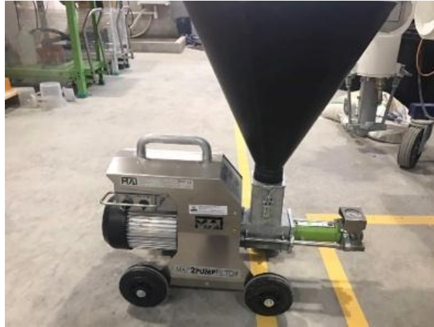
Fig. 7 MAI Pictor pump to convey materials
