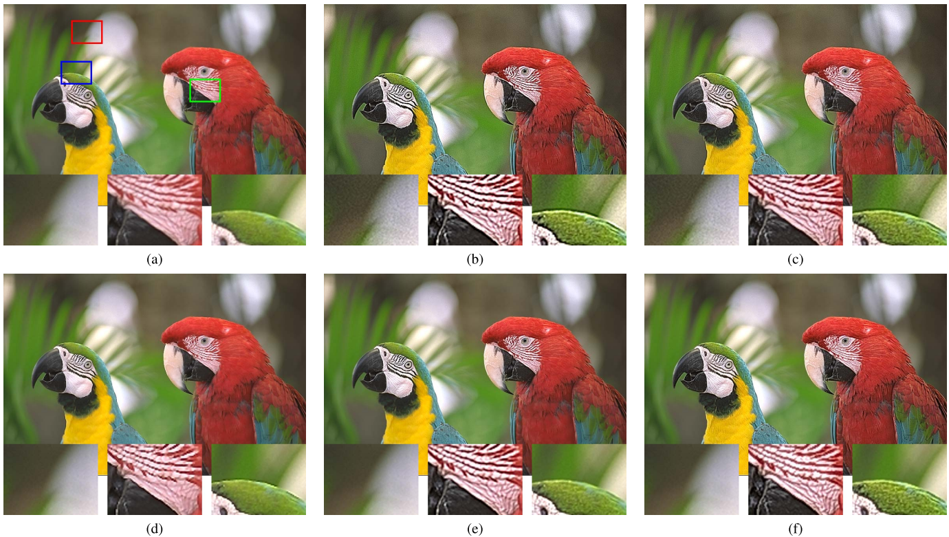
Fig. 7. Visual comparison of some enhancement results experimented on the test image “Parrot:” (a) the original image and its enhanced versions using the following methods; i.e., (b) the conventional UM with the Gaussian filter, (c) the modified GUM with the Gaussian filter [8], (d) the CUM [5] with the Laplacian filter, (e) the TUM [29] with the Gaussian filter, and (f) the proposed BUM with the Gaussian filter (when \eta = 1 ).
