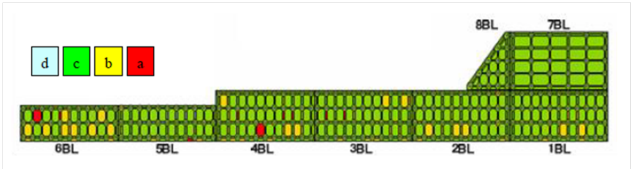
Figure 4. Inspected results of deteriorating grades for the concrete slabs in 2001
