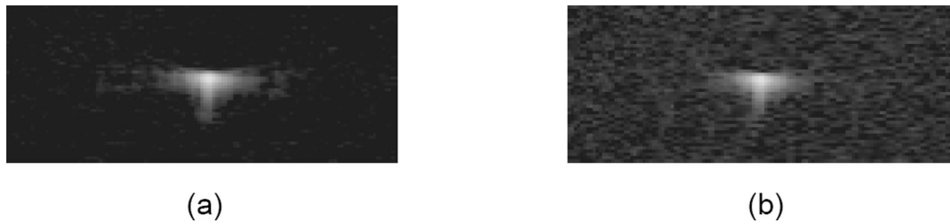
Fig. 1. Point phantom images: (a) without dynamic focusing artifacts and (b) with dynamic focusing artifacts.
