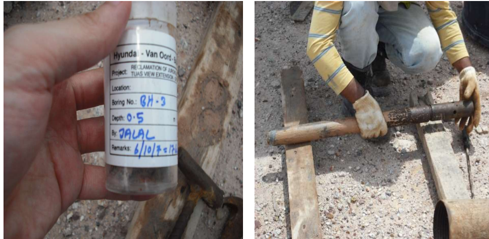
Figure 5.4 Sample retrieval from SPT test
