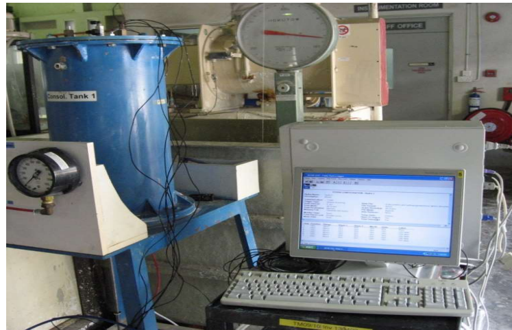
Figure 4.5 Physical set up of the cylindrical vacuum consolidation tank
