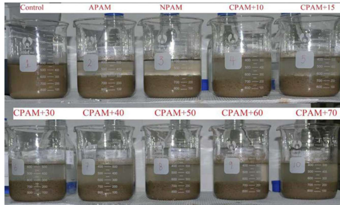
Figure 3.7 Sedimentation of dredged slurry mixtures using different PAM flocculants
