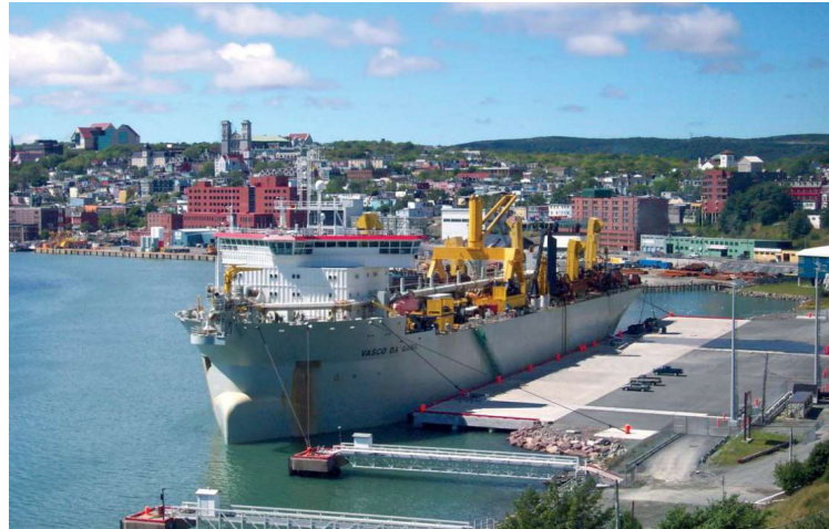
Figure 2.17 Relative size of 33,000m 3 mega TSHD Vasco Da Gama berthing at St John's Newfoundland (Fitzsimons, 2017)
