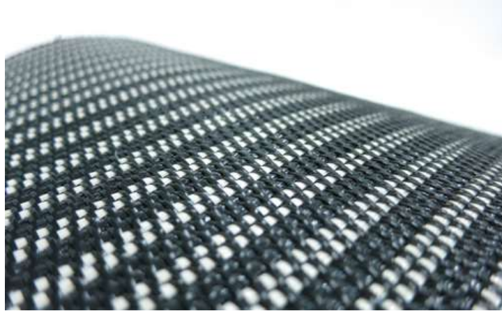
Figure 6.23 Woven fabric details of Mirafi HPa 380A
