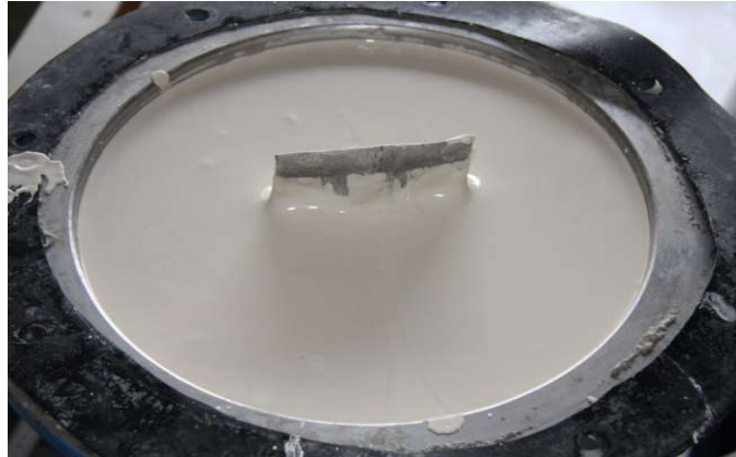
Figure 4.1 Kaolin slurry sample that represents dredged seabed slurry with high clay content
