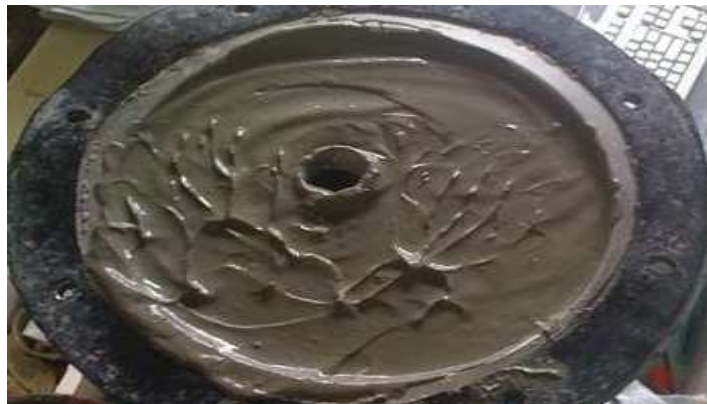
Figure 4.2 MC1 from Marina South seabed contain mainly Kallang Formation materials
