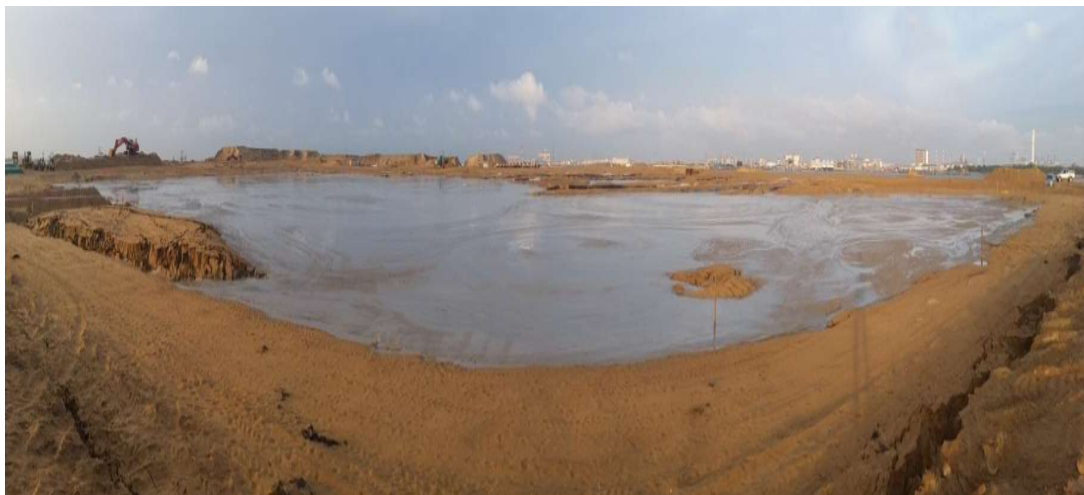
Figure 6.47 Photo showing the extend of the coverage of the slurry seepage on day
