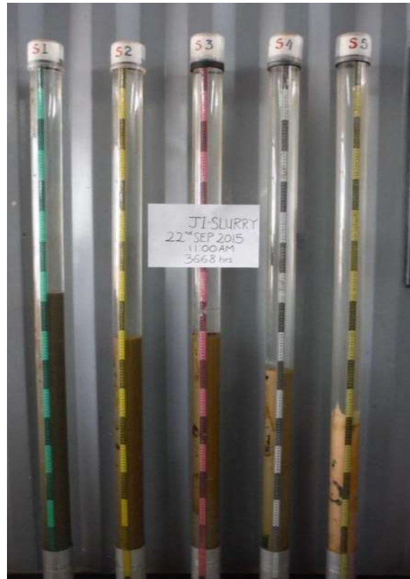
Figure 3.1 Photo showing the settlement of the columns at the 3668hrs
