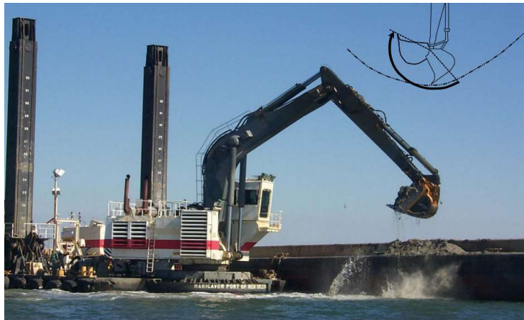
Figure 2.10 Scooping of seabed materials using backhoe dredger (Welp, 2006)
