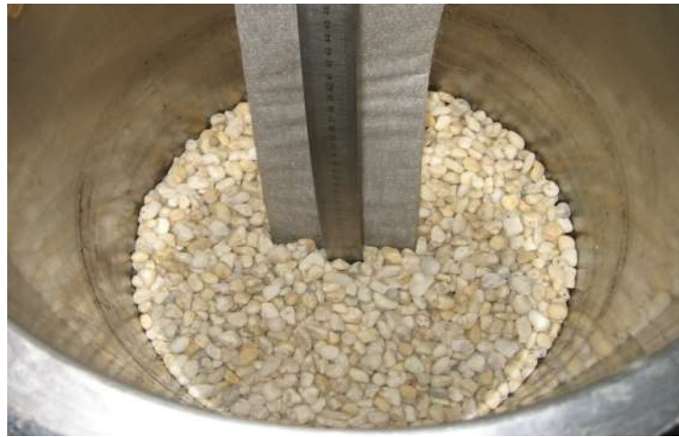
Figure 4.8 Gravel drainage layer for membrane vacuum consolidation technique
