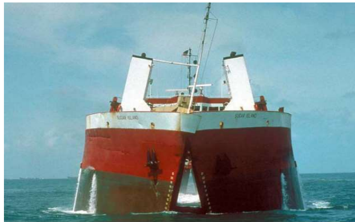
Figure 2.12 Split-bottom barge (US, 2015)
