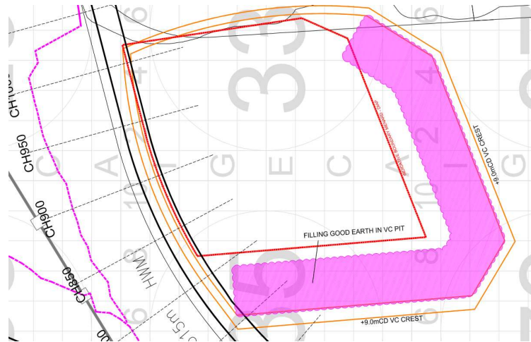
Figure 6.14 Good earth filling at the sides of the inner containment bund (pink)
