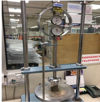
Figure 7.23 Unconfined compression test apparatus and a typical failed soil sample
