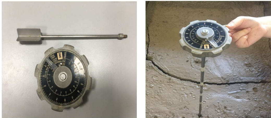
Figure 7.19 Pilocon hand vane tester used for undrained shear strength measurement
