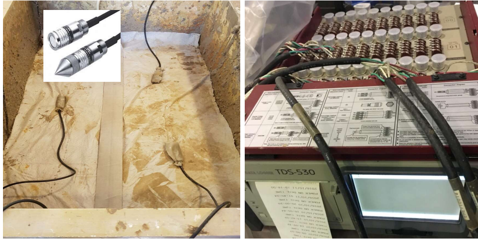
Figure 7.10 Pore water transducers and data logger used for model tests
