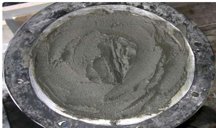
Figure 4.3 MC2 from Tuas seabed contain mainly Jurong Formation materials
