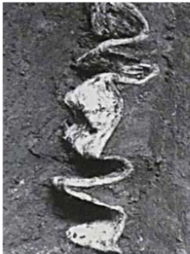
Figure 2.41 Folded PVD in soil with large settlement (Stapelfeldt, 2006)
