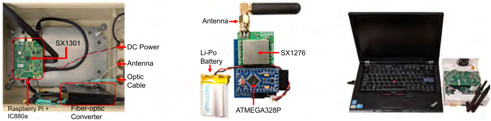
(a) The handcrafted LoRa gateway developed with IC880A front-end and Raspberry-Pi enabled processing unit.
