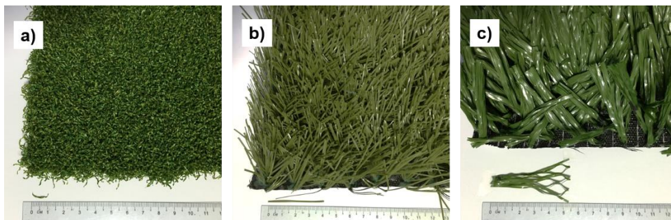
Figure 2.1. Examples of artificial turf carpets of various fibre types: a) 1G nylon, b) 2G monofilament short-pile and c) 3G fibrillated long-pile.
