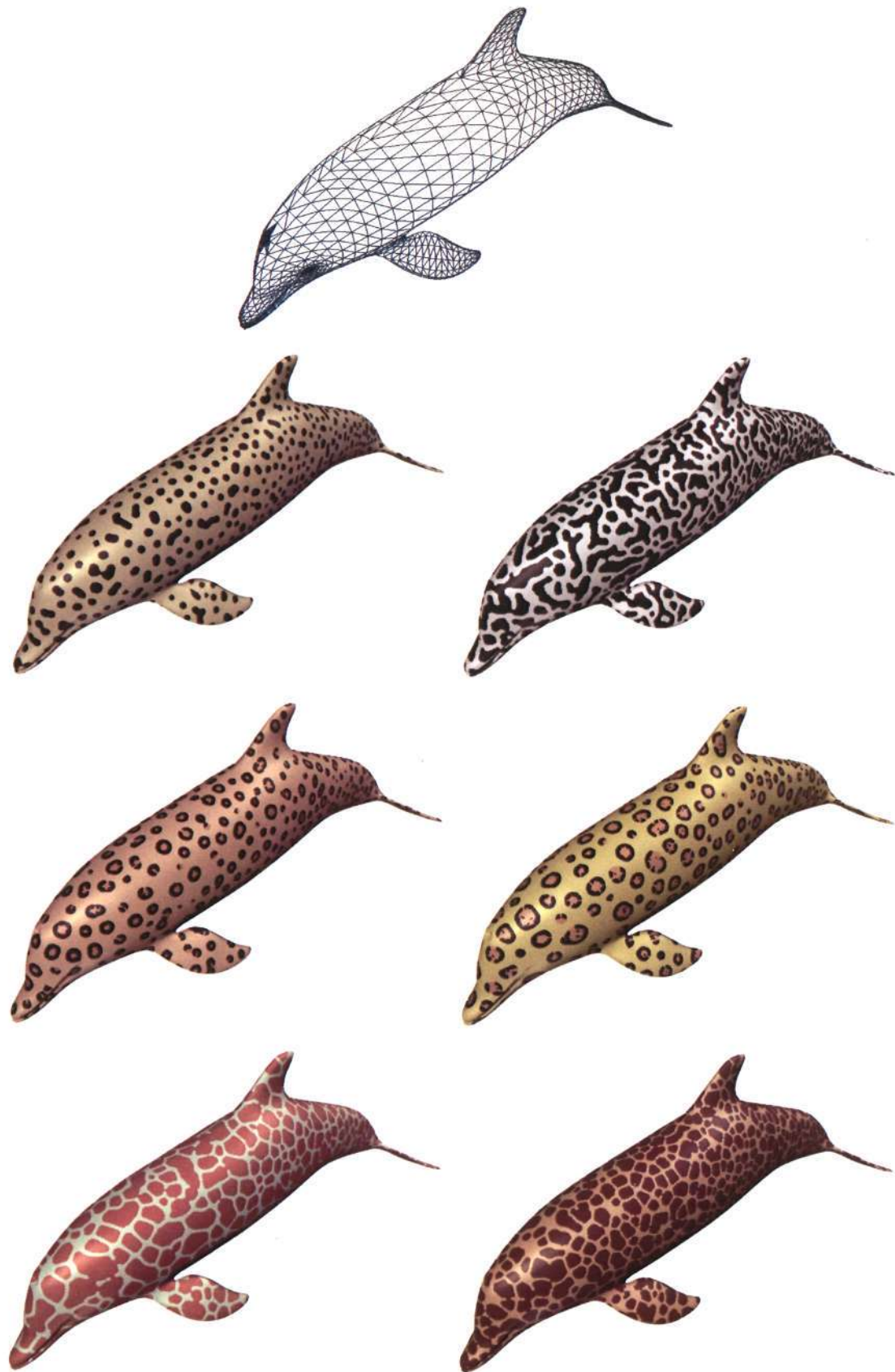
Figure 7.21: Dolphin model with 4198 triangles and simulated with 20000 cells
