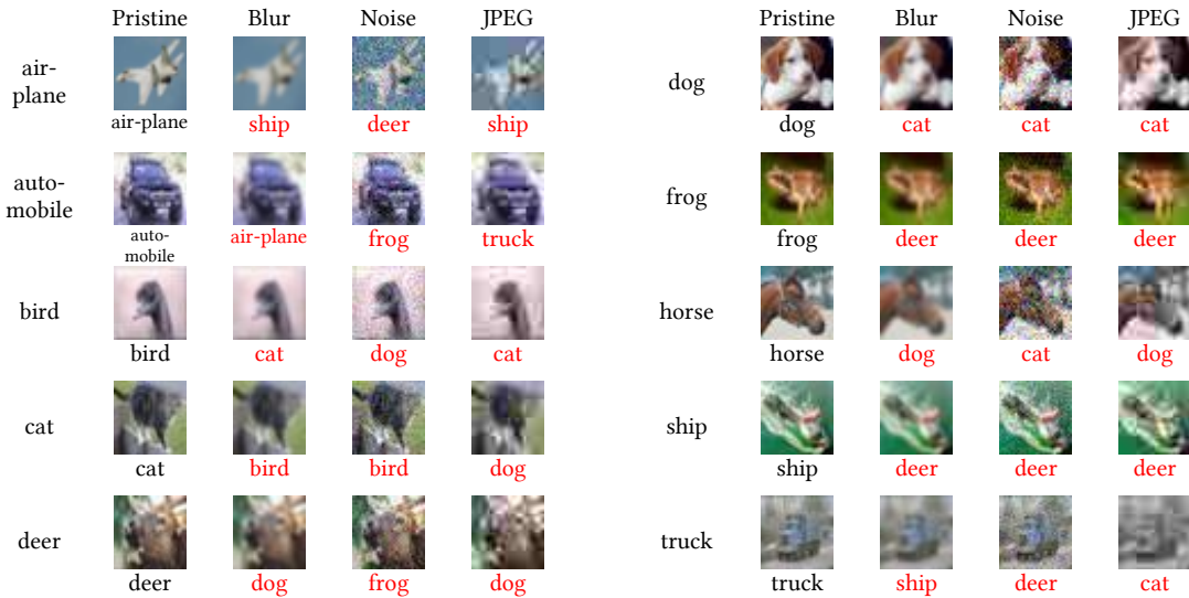
FIGURE 5.1: Illustration of the classification results of the 10 classes in CIFAR-10, where each class set including one pristine sample image and its corresponding distorted images. The first column of a class set is the pristine sample image of CIFAR-10. The second, third and fourth columns are the images corrupted by blur, noise and JPEG compression respectively. Given the pristine images, a DNN model can correctly identify them. However, when distortions are injected, the DNN model may misclassify the inputs. The labels below thumbnails are the prediction results by the DNN model.
