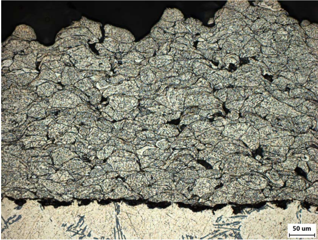
Figure 4.18b: SEM of Al-6061 coating which has been subjected to stress relief at 150 °C for 2 hours (200x magnification).
