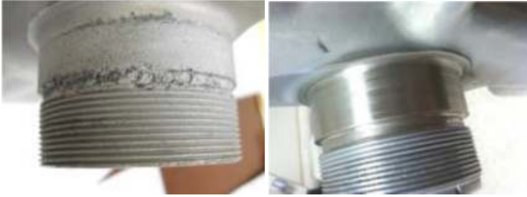
Figure 2.16: Before and after photos of cold sprayed repaired B737 nose wheel steering actuator barrel [MOOG Aircraft Group, 2012].
