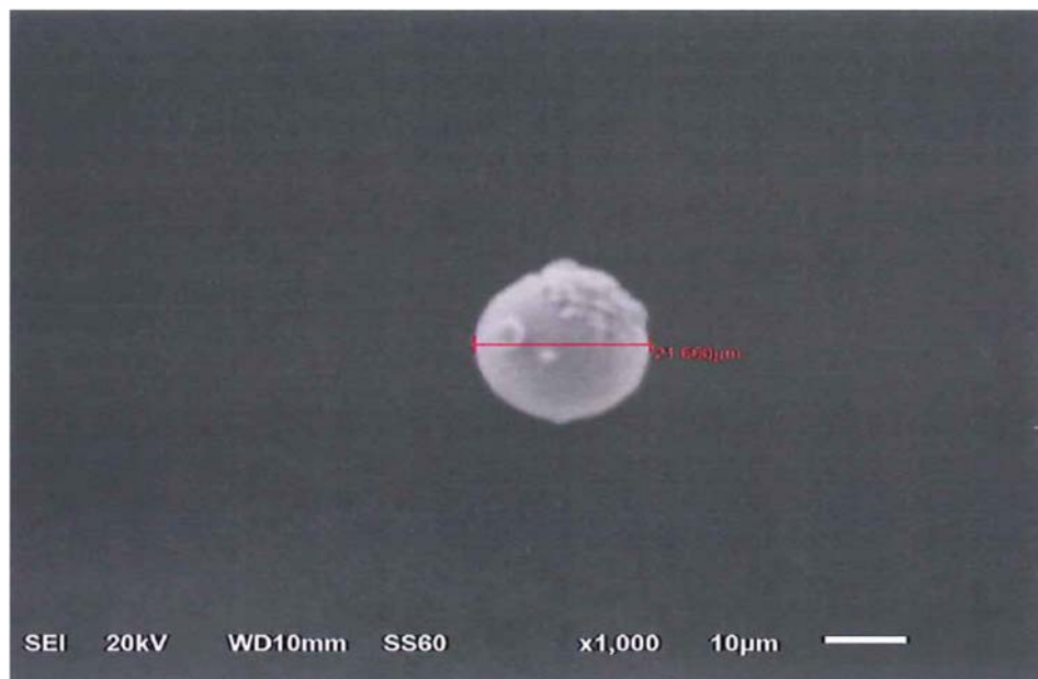
Figure 3.14a: SEM image of feedstock aluminium powder at 1000x magnification.
