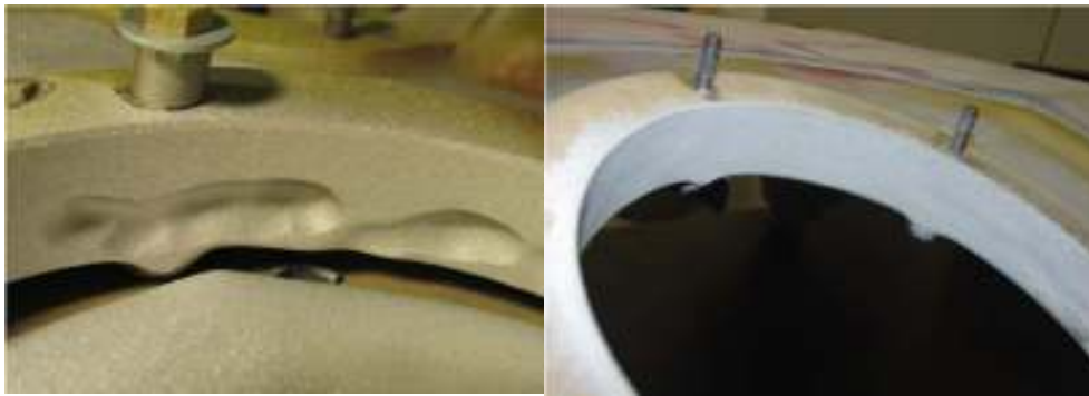
Figure 2.14: Magnesium helicopter transmission gearbox restored by cold spray using CP aluminium and Al-6061 aluminium alloy powders [Champagne, 2008].
