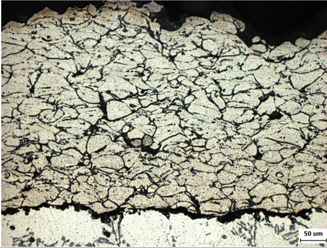
Figure 4.19b: SEM of Al-6061 coating which has been subjected to annealing at 535 °C for 2 hours followed by 177 °C for 8 hours (200x magnification).
