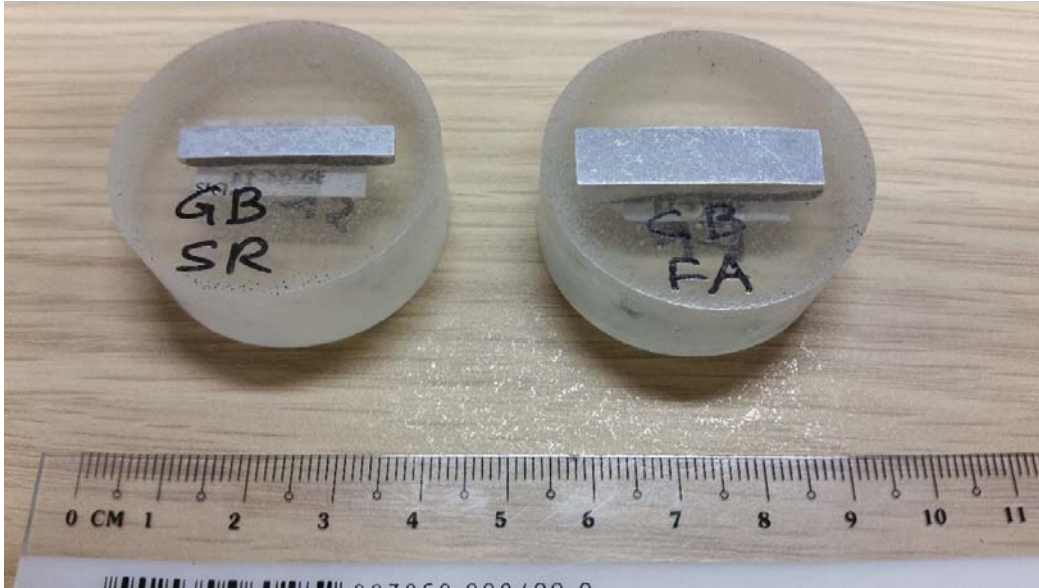
Figure 4.17: Cold sprayed coating samples which have undergone stress relief and full annealing sectioned and etched for microstructure evaluation.
