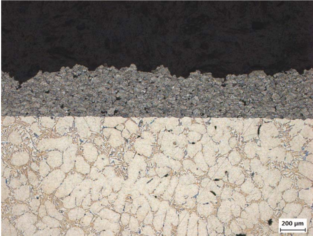
Figure 4.11a: SEM of Al-6061 coating on non-grit blasted substrate at 50x magnification.
