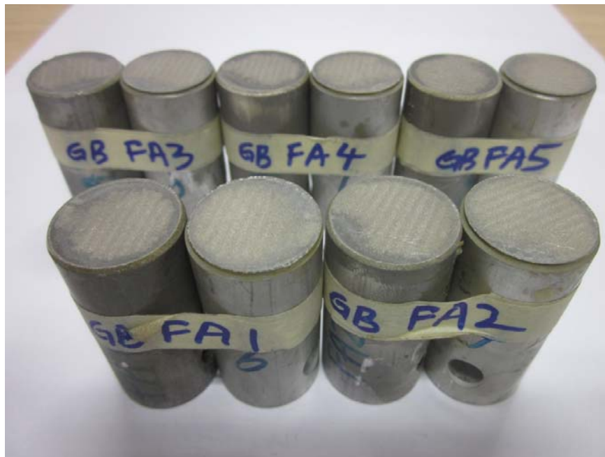
Figure 4.15b: Adhesion strength test specimen with cold sprayed coating which has undergone annealing.
