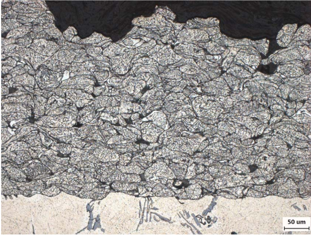
Figure 4.11b: SEM of Al-6061 coating on non-grit blasted substrate at 200x magnification.
