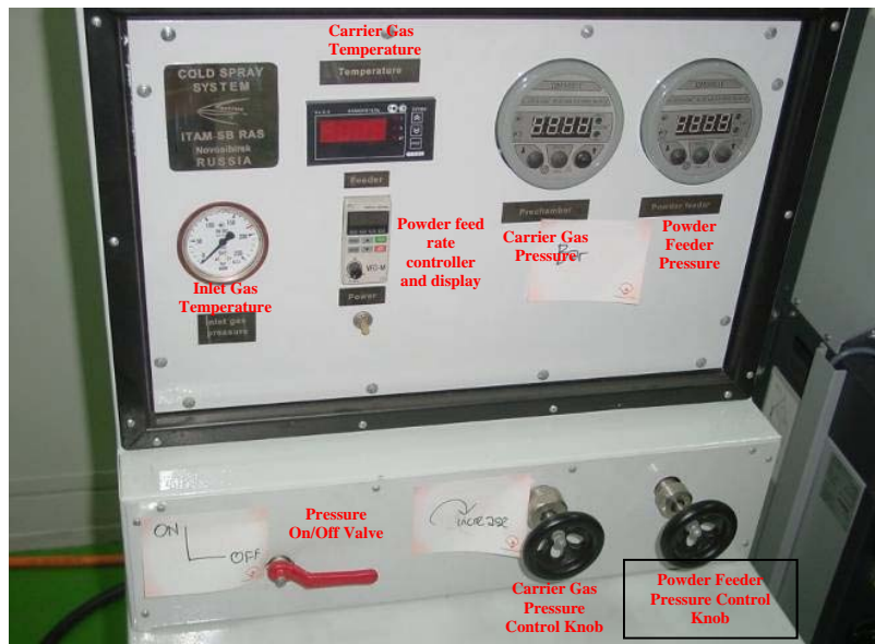
Figure 3.6: Cold spray system control panel.
