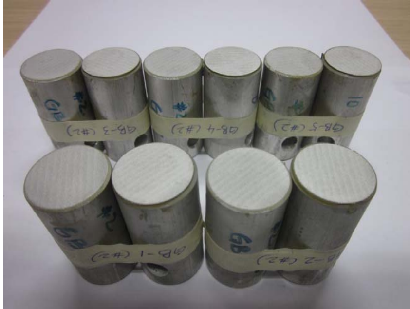
Figure 4.8a: Adhesion strength test specimen with coating cold sprayed on grit blasted substrates.
