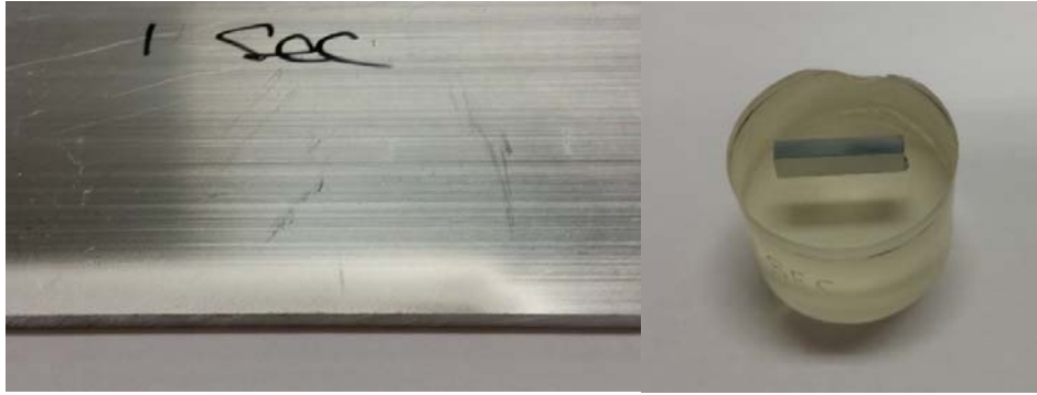
Figure 6.4b: Al-6061 cold spray coating obtained with the nozzle held stationary for one second was sectioned, mounted, etched and polished for microscopic evaluation.
