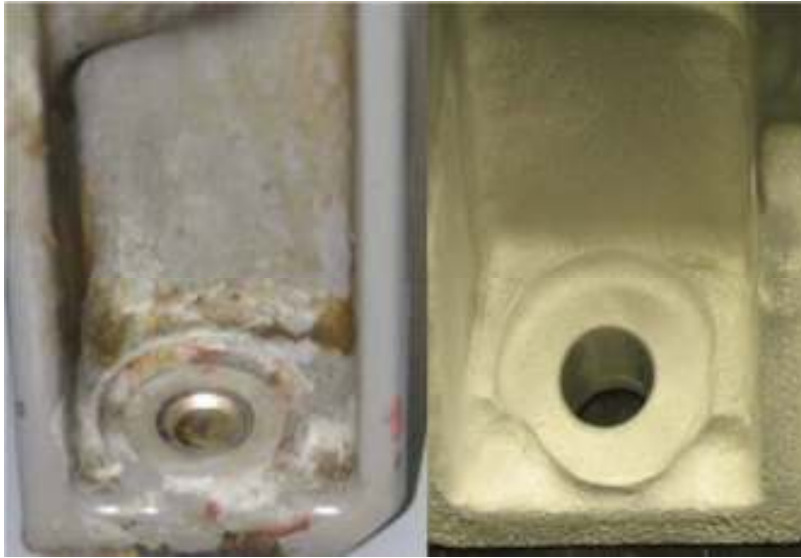
Figure 2.15: Restoration work on UH-60 main rotor transmission housing using cold sprayed CP Aluminium and Al-6061 Aluminium powders [Champagne et al. , 2012]
