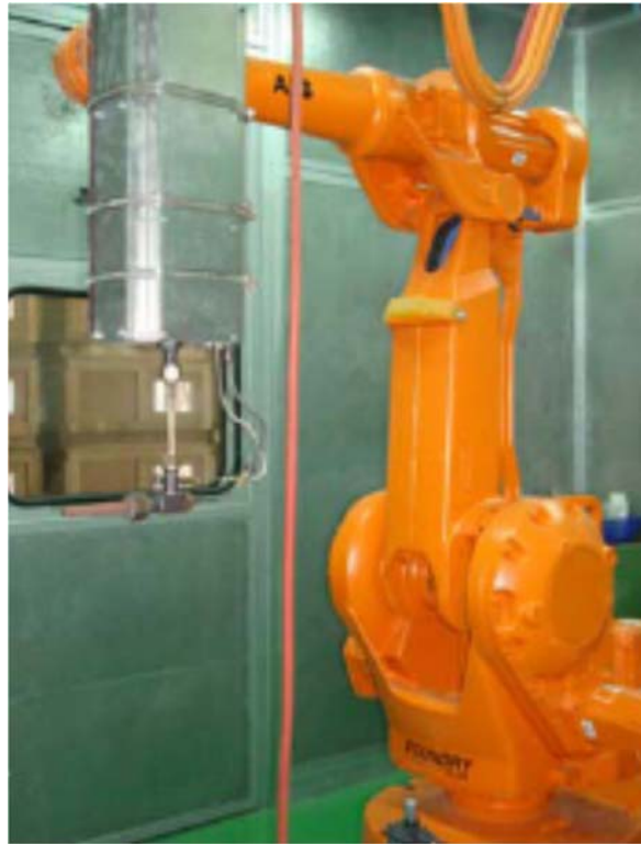
Figure 3.7: ABB IRB 2400 robot with cold spray gun and gas heating device mounted.
