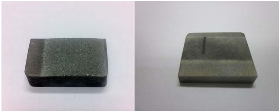
Figure 4.13: Al-6061 cold spray coated specimen which has undergone (a) stress relief and (b) full annealing.
