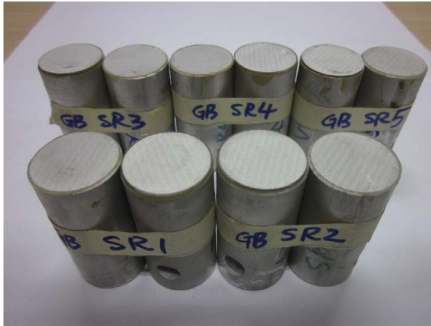
Figure 4.15a: Adhesion strength test specimen with cold sprayed coating which has undergone stress relief.
