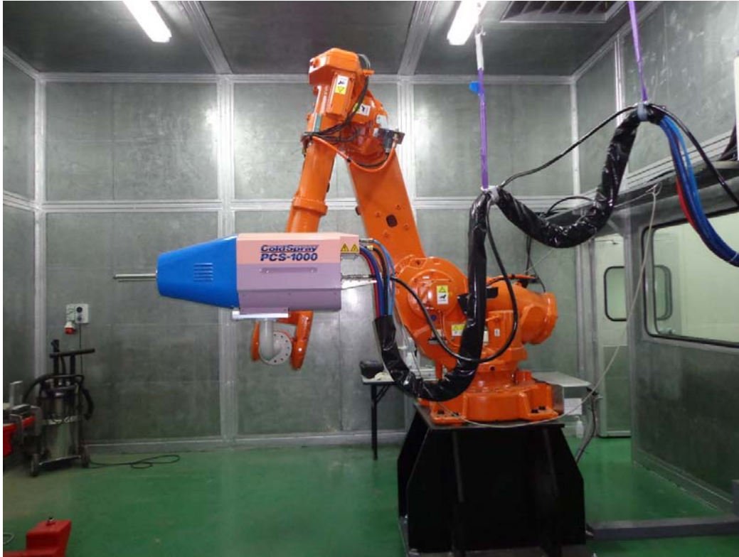
Figure 3.8b: Spray room for new PCS-1000 cold spray system.
