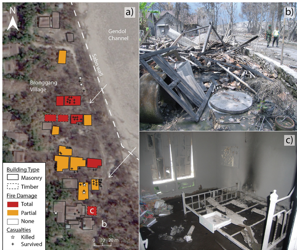
Fig. 5. a) Spatial distribution of building type, fire damage and casualties in a section of Bronggang village (inset in Fig. 2), ~13.5 km from the summit and subject to LEDS. LEDS flow direction across sabo walls is indicated by white arrows with the white dashed line marking the sabo concrete levees bordering the Gendol channel, b) remains of a burned and charred timber-framed building that was totally destroyed by fires caused by LEDS (Photo taken by S.F. Jenkins 28 days after impact on 3 December 2010), c) straw mattress burned by an isolated fire as a result of LEDS inundation (Photo taken by S.F. Jenkins 29 days after impact on 4 December 2010). The location of the images in (b) and (c) are marked by the corresponding letters in (a).
