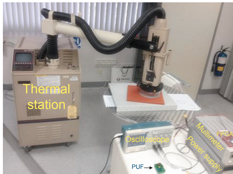
Figure 4.17: The probe station for the testing of the sample chips.
