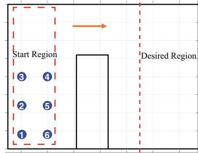
Fig. 6 Schematic diagram of the flight area and initial positions of drones. The six drones are placed in the flight area and the initial position of the informed agent can be selected by one of the six positions
