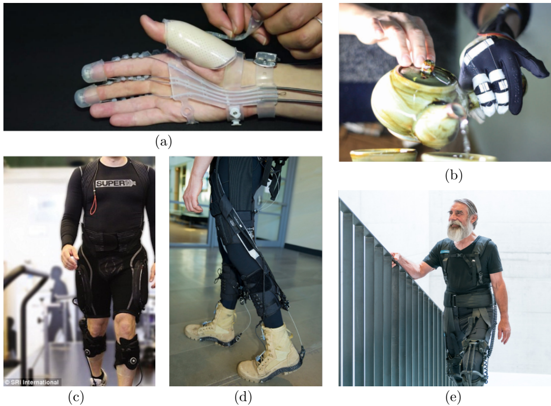
FIGURE 2.5: Tendon-driven soft exosuits. (a) The Polyglove is a silicone-based wearable robot that uses a Bowden cables and a flexible structure to assist SPI patients in grasping. (b) The same group developed a fabric-based glove to achieve the same goal. (c)-(d)-(e) The Superflex from SRI, the exosuit from the Wyss Institute at Harvard and the Myosuit from Myoswiss, shown from left to right, all use electric motors, driving tendons routed in the fabric, to assist locomotion.
