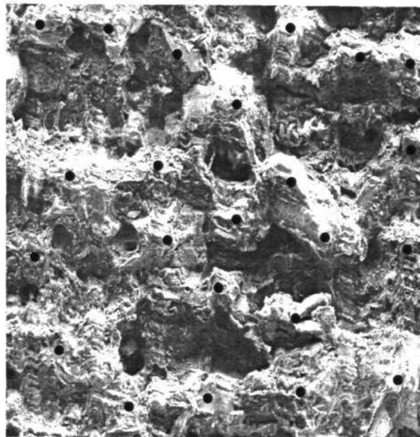
Figure 4.7 Topography of B120H200V grinding wheel sample, obtained with (a) stylus system, (b) SEM. The dot marks an abrasive grain by using the “eight nearest neighbour” summit definition (stylus) and visual inspection (SEM). The sampling interval is 60\ \mu\text{m} ( 0.37S_{al} ). Line “—” marks a deep valley that the stylus tip could not access. Line “---” marks an omitted grain
