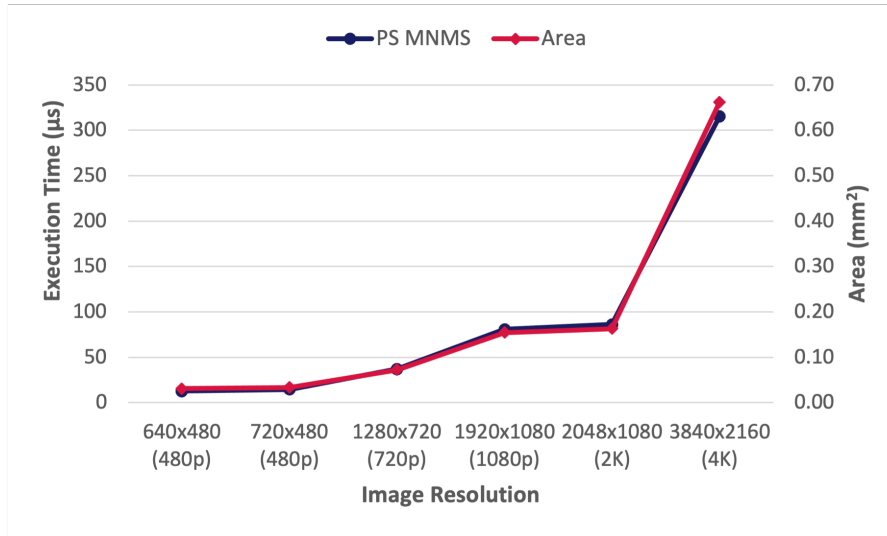
FIGURE 4.20: The execution time of PS MNMS, the capacity of SMM, and the area in varied image resolutions that is supported by an 8-bit 1-way 1-bank ShapoolNMS at 400 MHz. The data transferring time between GPUs or deep learning accelerators and ShapoolNMS is hidden by the Relationship Recovery process time.
