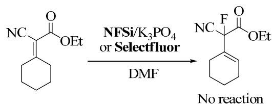
Scheme 2.3.6 Electrophilic Fluorination of \alpha -cyano- \alpha -carbonylolefin with Selectfluor or NFSi/Base System
