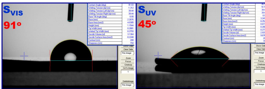
Figure 7-5 Water contact angle of the photo-responsive smart surface in the cases under S_{VIS} and S_{UV} , respectively.
