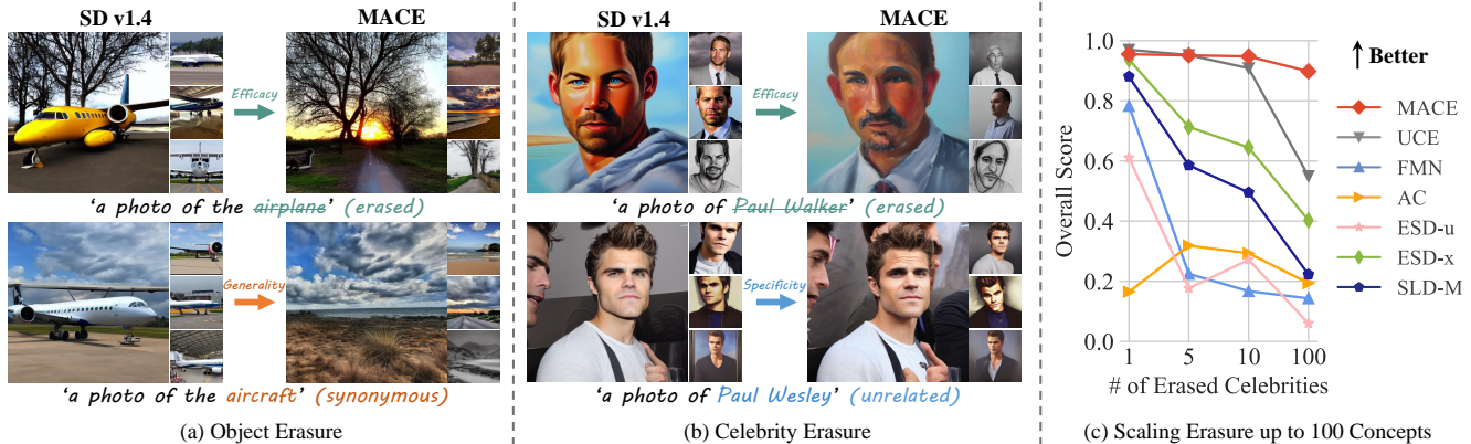
Figure 1. Our proposed method, MACE, can erase a large number of concepts from text-to-image diffusion models. This can safeguard celebrity portrait rights, respect copyrights on artworks, and prevent explicit content creation. (a) MACE demonstrates good efficacy and generality by preventing the generation of images reflecting the target concept and its synonyms . (b) MACE maintains excellent specificity, ensuring that the unintended concepts remain intact, even when they share common terms with the target concept . (c) MACE exhibits a significantly enhanced ability to erase 100 concepts, outperforming previous methods. The overall score indicates the comprehensive erasing capability, as detailed in Section 4.3.
