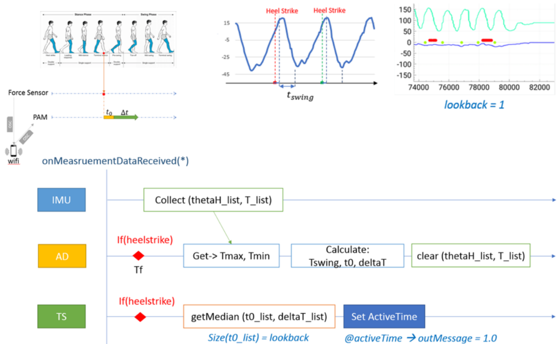
Figure 6.2: Automatic Controller Implementation
