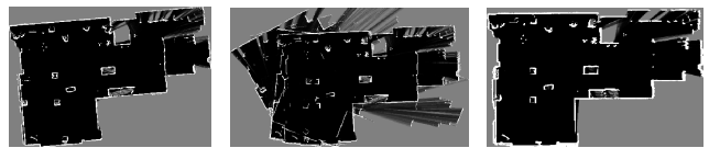
(a) HectorSLAM at (b) HectorSLAM at 0.8m/s (c) UWB/LiDAR at 0.8m/s 0.4m/s
