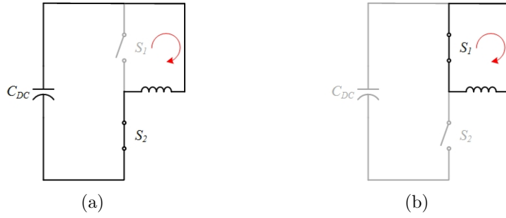
Figure 7.2: Operation principle of chopper: (a) S_1 off and S_2 on, (b) S_1 on and S_2 off.
