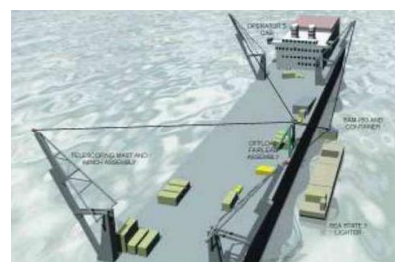
(b) Diagram of the Cable Array Robot used for loading containers onto a ship [20]
