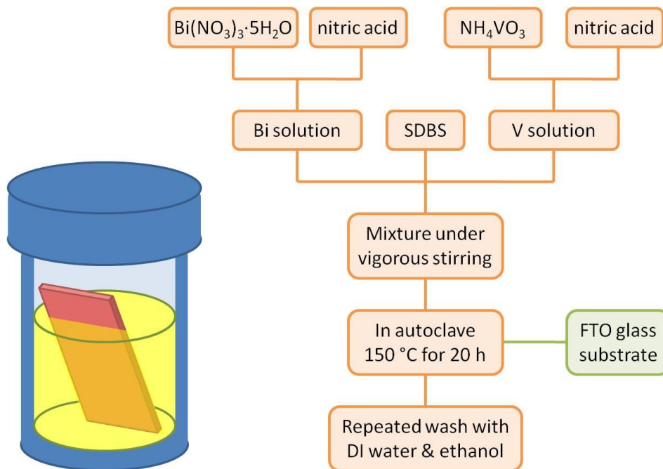
Figure 8.5 Schematic illustration and procedure of m\text{-BiVO}_4 film preparation by hydrothermal chemical bath deposition.
