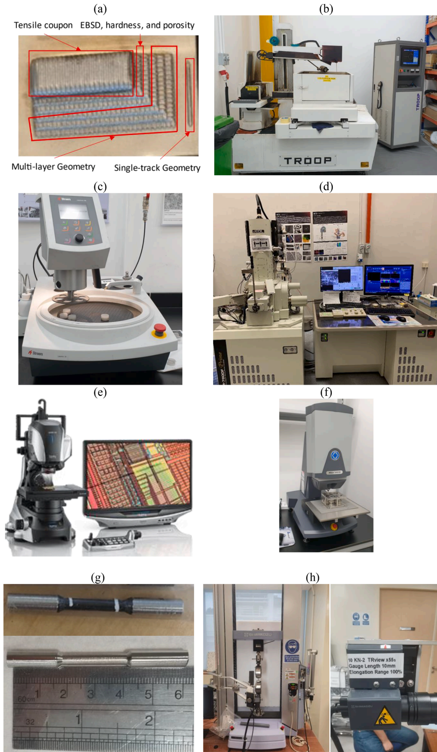
Fig. 3. Sample preparation (a) printed part, (b) Troop wire cut machine, (c) Struers Tegramin 25, (d) JOEL FESEM 7800F, (e) Keyence VHX-7000, (f) Wilson-VH3100, (g) tensile coupon, (h) Shimadzu tensile tester.
