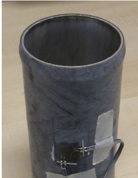
Figure 8: Bulging at one end of a composite pipe specimen after axial compression test
