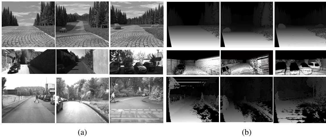
Fig. 3.8 Samples of three datasets for road surface detection: (a) left images of the stereo pairs from the enpeda dataset (first row), the KITTI dataset (second row), and the Daimler dataset (third row) and (b) their corresponding disparity maps for the three datasets used in the experiments. The contrast is enhanced for better visualization. The disparity maps serve as the inputs.
