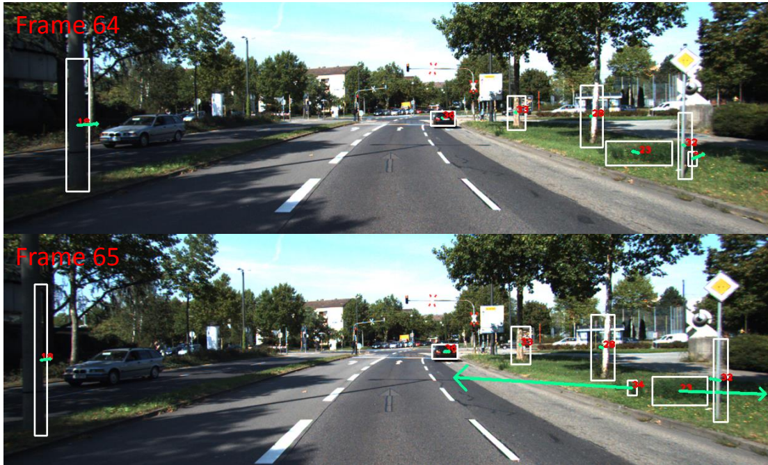
Fig. 6.13 Typical failure case II: some bushes appear on the right side of the road and are detected with tracklet id 23 and 34. Since the corresponding disparity map for this part is not accurate, the detected range for them are not accurate. Hence, motion is detected for them, even though they are in fact stationary.
