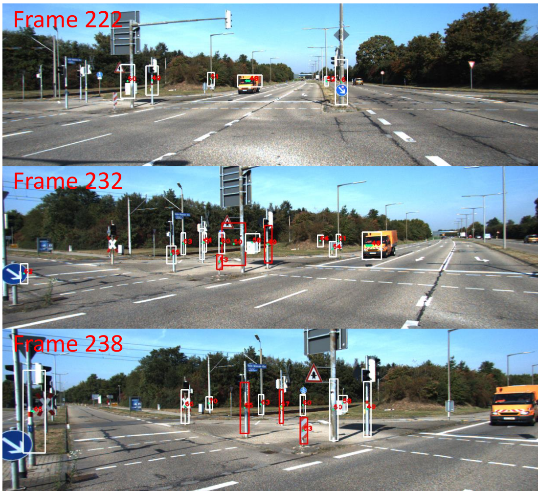
Fig. 6.14 Typical failure case III: Taking the assumption that ego-vehicle will keep its motion state unchanged in near future, collision risk for obstacles with id 49 and 50 is predicted at frame 232 since they are located in the predicted course of the ego-vehicle at that moment. However, the ego-vehicle is in fact making a left-turn and obstacles with id 49 and 50 should not pose any collision risks.
