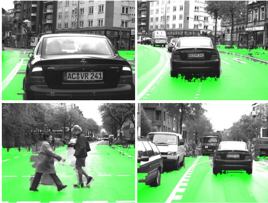
Fig. 3.12 Examples of the detection results of the proposed algorithm for scenarios where the vicinity of the vehicle is filled with crowded objects.
