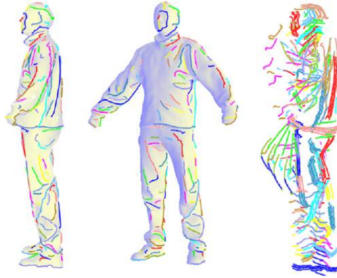
Figure 5.2: An example of Crane model rendered with 3D paths traced from ridges and valleys extracted from current view (left) and another view (middle). The overlapping 3D paths show their evolution during the animation (right).
