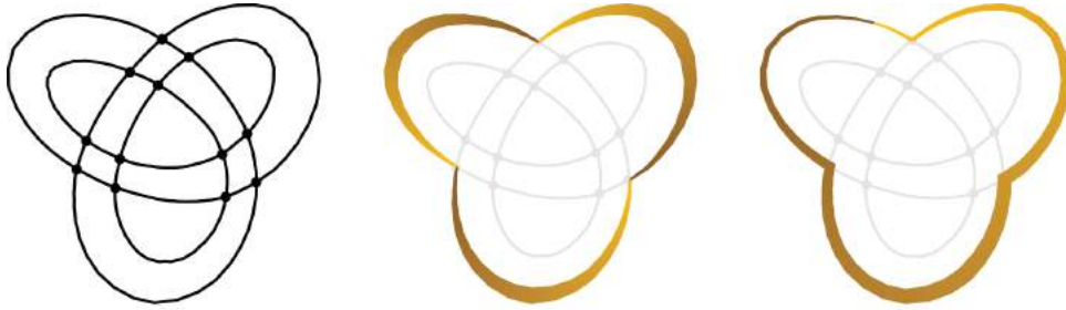
Figure 2.18: Stroke topology (images courtesy of Grabli et al. [39]). A planar graph (left). Middle and right show the same path in the graph drawn with the same low-level attributes but with three strokes and one stroke respectively.
